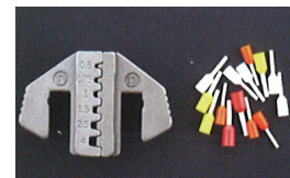
D DIE Cord End Terminal AWG 22/20/18/16/14/12 0.5/0.75/1.0/1.5/2.5/4.0 mm 2
