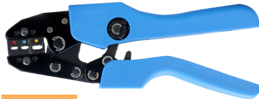
KC-8A For Insulated Terminal & Connector AWG 20-18/16-14/12-10 0.5-1.0/1.5-2.5/4.0-6.0 mm 2
