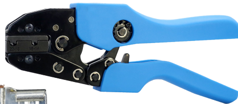
KC-8FL02 For Non-Insulated 90° Flag Terminal AWG 20-18/16-14 0.5-1/1.5-2.5 mm 2
